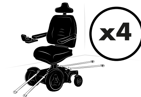
Figure 1.57. The wheelchair has four tie-down points. The wheelchair and tie-down position in this picture is generic.
