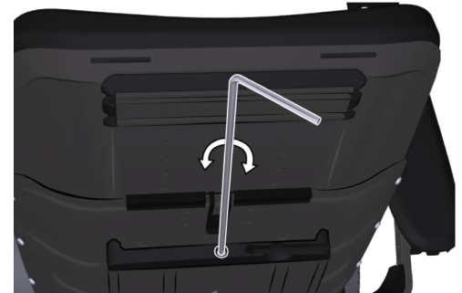
Figure 126. Use the supplied adjustment crank.
