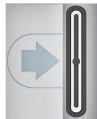
Figure 35. Right turn signal button and screen symbol.
