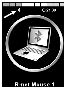
Figure 53. The arrow points to the flashing Bluetooth® icon.
