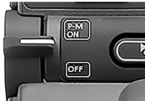
Figure 26. Power, mode and profile paddle.
