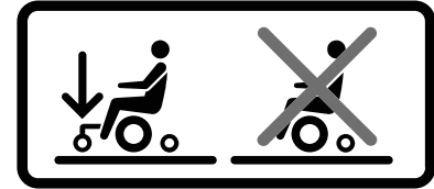
Figure 6. The support wheels must always be fitted when you drive.
