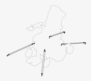
The wheelchair shall be forward-facing when you use it as a seat in a vehicle. Permobil has no manufacturer-designated wheelchair-mounted belt restraints. Use the vehicle's restraint systems.
