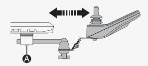
This is how you adjust the resistance of the rotational panel holder. Loosen or tighten the knob  $\bullet$  on the friction joint to adjust how easily the rotational panel holder can be pushed to either side.
