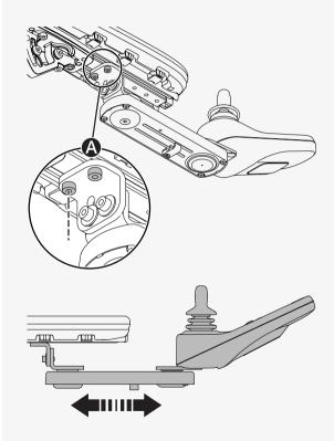
This is how you adjust the angle of the control panel.
