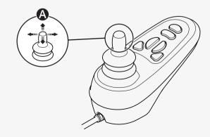
Drive as gently as possible and avoid sudden braking. Do not turn off the power to stop the wheelchair. If you turn off the power while you drive, the wheelchair will stop abruptly.
