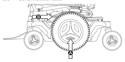
The serial number label is located on the lower, left side of the wheelchair chassis **3**. An additional serial number label is located on the seat tilt **3**. You may need to tilt the seat to see the serial number label.
