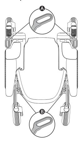
The wheelchair is equipped with four tie-down points used for transportation  $\rightleftharpoons$  **X**  $\rightleftharpoons$ . Two in the front  $\spadesuit$  and two in the rear  $\circleddash$ .
