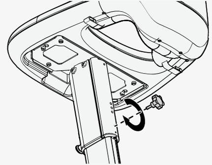
2. Remove the tightening knob from the column.
