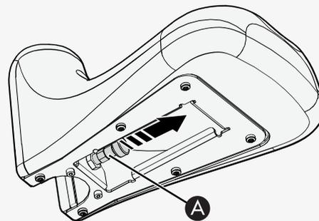
4. Push the seat into the groove on the column.
