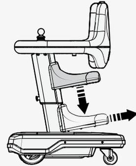
5. Put back the tightening knob and tighten it by hand.
