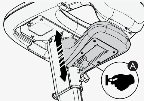
2. Remove the tightening knob (A) from the column.
