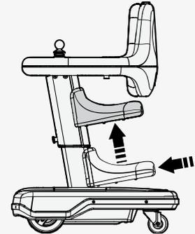
6. Release the plunger knob (A). A click signals that the plunger knob is locked.
