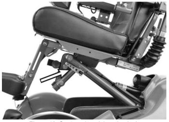
Figure 12. Seat angle quick-acting lock.
