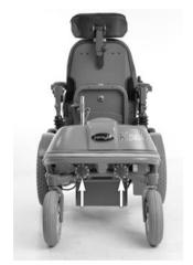
Figure 4. Rear Lights and Reflectors.
