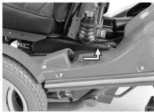
Figure 88. Brake release lever.
