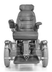
Figure 3. Front Lights and Reflectors.
