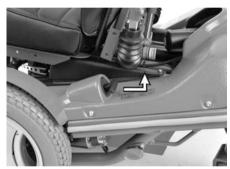
Figure 93. Brake release lever
