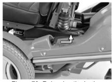
Figure 79. Releasing the brakes
