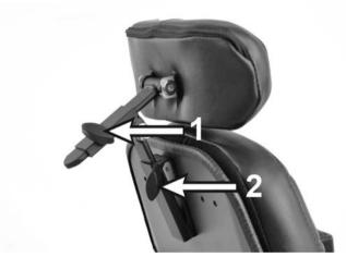
Figure 19. Head rest adjustment
