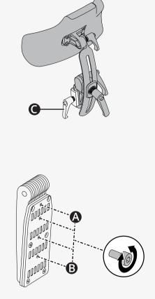
This is how you adjust the height and depth of the headrest.  $\checkmark$  Allen key 5 mm
