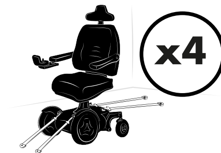
Figure 131. The wheelchair has four tie-down points. The wheelchair and tie-down position in this picture is generic.
