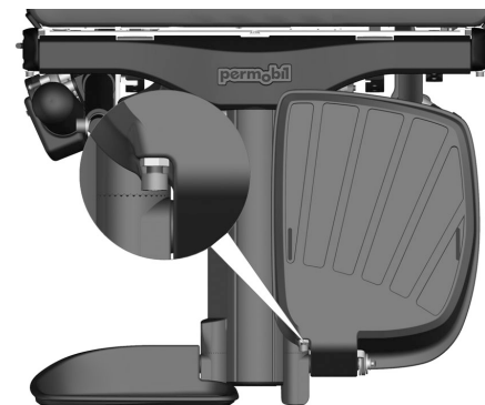
Figure 107. The angle of the foot plates can be adjusted using a screw locked with a lock nut
