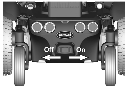
Figure 144. Resetting the main fuse
