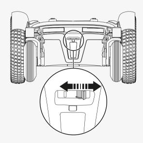
When you store it for a long time, fully charge the batteries before storage. Remember to switch off the main circuit breaker. Charge the batteries every month. You will need to switch on the main circuit breaker to charge the batteries, then switch off the main circuit breaker if the wheelchair is to remain in storage.
