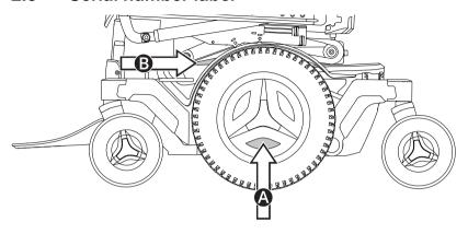
The serial number label is located on the lower, left side of the wheelchair chassis. Look between the rim spokes **a**. An additional serial number label is located on the seat tilt **a**. You may need to tilt the seat for better visibility.
