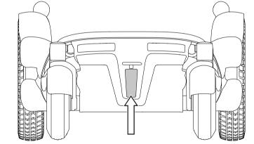
The wheelchair is equipped with reflectors at the front and rear.
