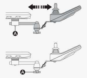
You can angle the rotational control panel to either side. This is how you adjust the angle.
