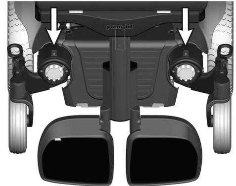
Figure 43. Location of the release levers
