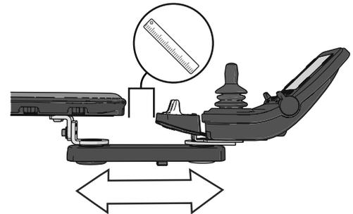
Figure 38. Adjusting the position on the parallel panel holder.
