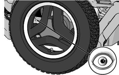
Figure 9. Chassis identification number label.
