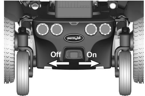
Figure 69. Resetting the main fuse
