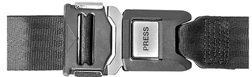
Figure 42. Belt buckle locked properly in the snap lock.
