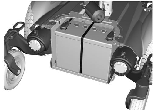
Figure 65. Front battery terminals
