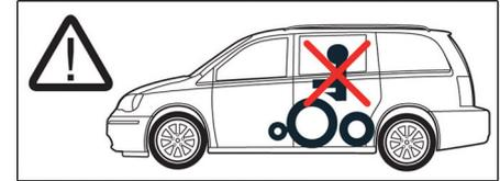
Figure 6. Use as seat in motor vehicle prohibited
