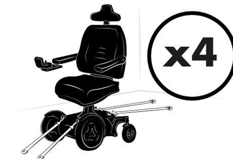
Figure 56. The wheelchair has four tie-down points. The wheelchair and tie-down position in this picture is generic.
