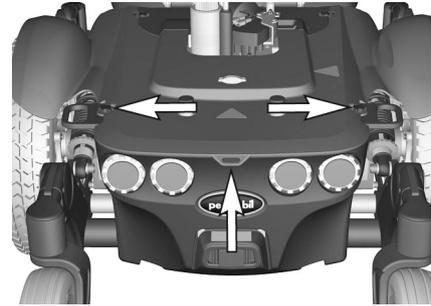
Figure 62. The rear cover is fitted together with the upper chassis cover
