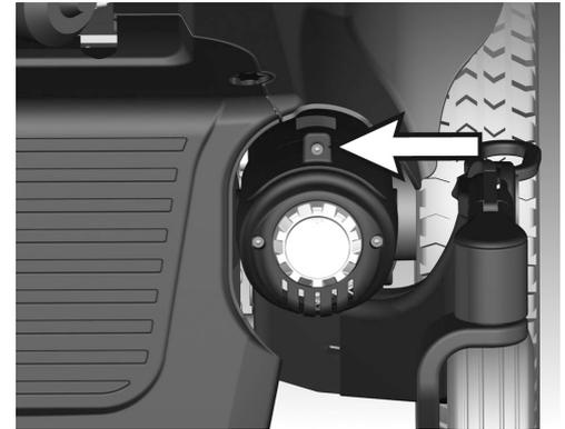
Figure 45. Wheel lock engaged
