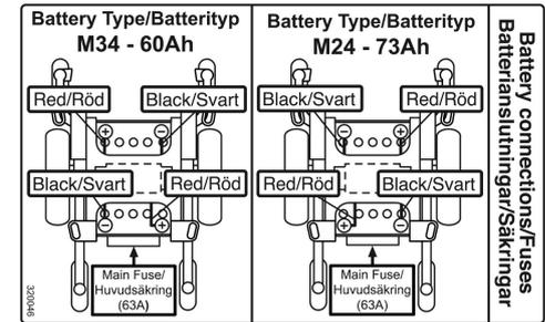
Figure 8. Battery connections and fuses
