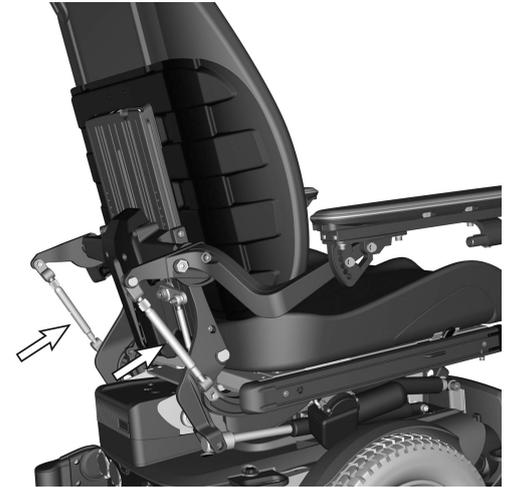
Figure 29. Adjusting the arm rest angle
