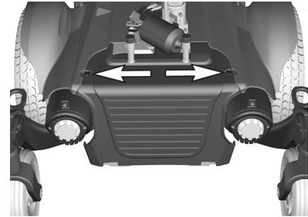
Figure 61 . Knobs holding the front cover
