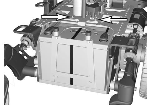
Figure 64. Rear battery terminals. The seat support is mounted with two screws
