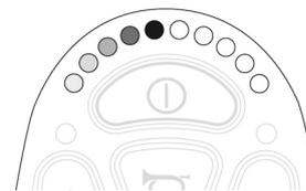
Figure 53. The LEDs on the battery voltage indicator.
