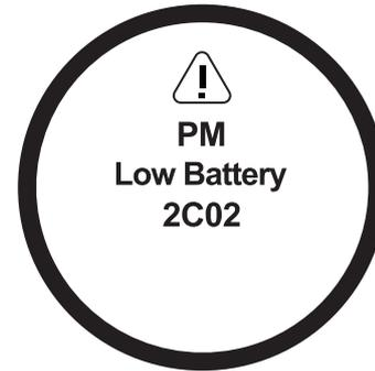
Figure 71 . Screen showing system fault indication.
