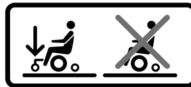
Figure 6. The support wheels must always be fitted when you drive.
