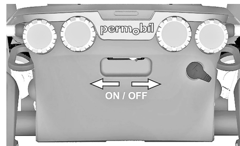
Figure 200. Main circuit breaker located under the Permobil logotype on the rear cover.
