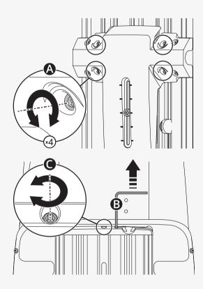
This is one way to adjust the angle of the armrest. The lower lock nut has a left-hand thread.
