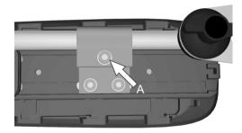
Figure 34. Screw for adjusting the panel holder length
