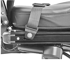
Figure 41. Attaching the positioning belt
