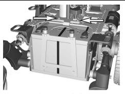
Figure 64. Rear battery terminals. The seat support is mounted with to screws
