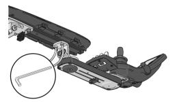
Figure 37. The position of the screws on the parallel panel holder.
