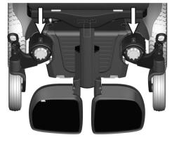
Figure 43. Location of the release levers
