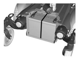
Figure 65. Front battery terminals
