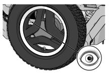
Figure 9. Chassis identification number label.
