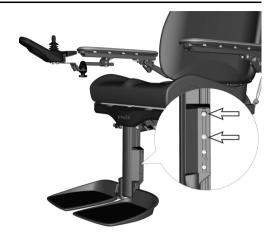
Figure 31. The height of the footplates is secured using the outer locking screws
