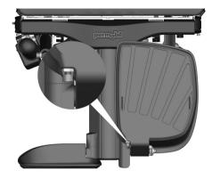
Figure 32. The angle of the foot plates can be adjusted using a screw locked with a lock nut
