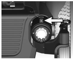
Figure 45. Wheel lock engaged
