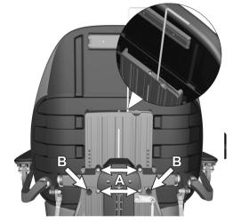
Figure 28. Adjusting the arm rest height
