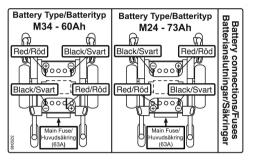
Figure 8. Battery connections and fuses
