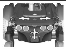
Figure 62. The rear cover is fitted togather with the upper chassis cover
