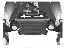
Figure 61. Knobs holding the front cover
