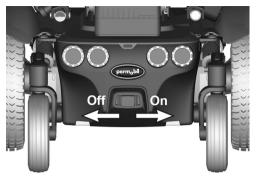
Figure 69. Resetting the main fuse
