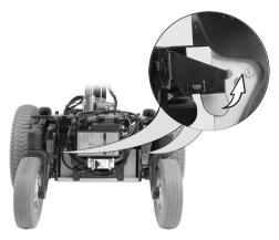
Figure 63. Remove the electronics by gently pulling the locking handles on the left and right side of the chassis outwards and disengaging the tabs
