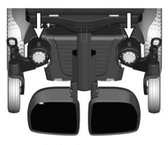
Figure 70. Brake release lever.
