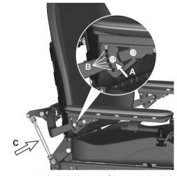
Figure 30. Individual adjustment of the arm rest height/angle
