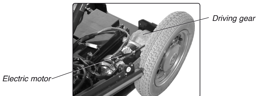
Fig 6. Electric motor with driving gear.
