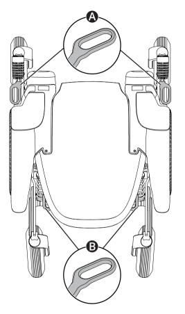
The wheelchair is equipped with four tie-down points used for transportation  $\blacksquare \checkmark \boxdot$ . Two in the front O and two in the rear O.
