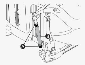
This is the other way to adjust the angle of the armrest. ≁ Allen key 5 mm
