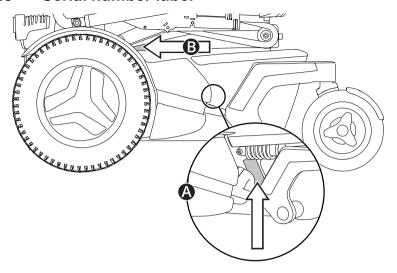
The serial number label is located on the lower, left side of the wheelchair chassis, see ②. An additional serial number label is located on the seat lift, see ③. You may need to lift the seat for better visibility.
