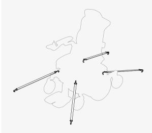
You must use both pelvic-belt restraints and shoulder-belt restraints. Make sure that the belt restraints are as tight as possible, without becoming uncomfortable, and that they are not twisted. They must be close to your body and not held away by parts of the wheelchair. Adjust your restraint system such that the release mechanisms cannot be pressed during a crash.
