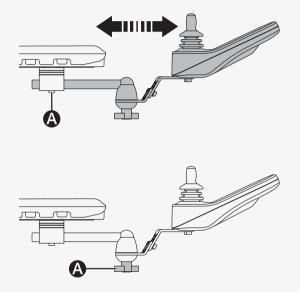
You can angle the rotational control panel to either side. This is how you adjust the angle.
