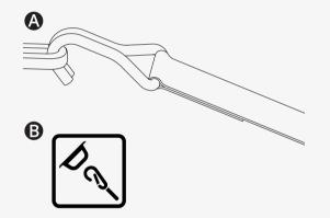
After you have secured the straps to your wheelchair, secure the other end of the straps to your vehicle according to the appropriate instructions. The end-fitting on the strap must comply with ISO 10542–1:2012, which is an international standard that governs wheelchair tie-downs and occupant-restraint systems. Every vehicle tie-down system is different, and it is important that you follow the instructions for your particular vehicle system.
