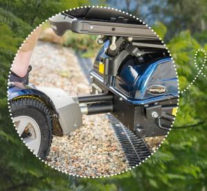
Powered extendable wheelbase provides enhanced stability for travelling over rugged terrain.
