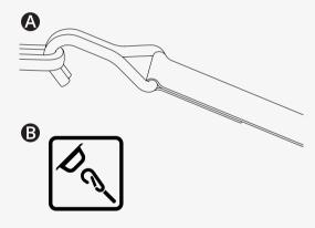
After you have secured the straps to your wheelchair, secure the other end of the straps to your vehicle according to the appropriate instructions. The end-fitting on the strap must comply with ISO 10542–1:2012, which is an international standard that governs wheelchair tie-downs and occupant-restraint systems. Every vehicle tie-down system is different, and it is important that you follow the instructions for your particular vehicle system.
