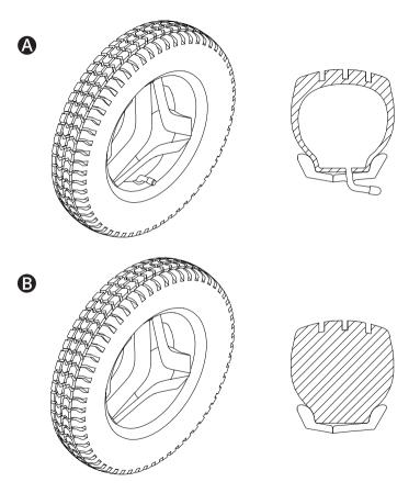
The wheelchair drive wheels have pneumatic tires or flat-free (foam filled) tires. The caster wheels have pneumatic tires or solid polyurethane tires.
