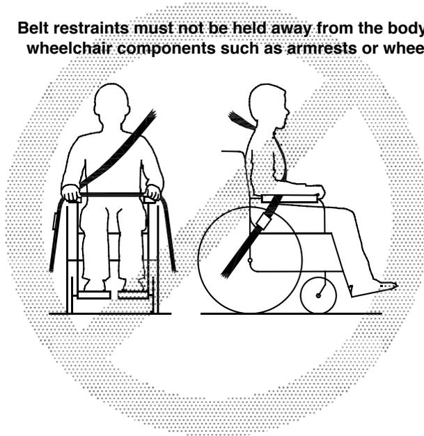
6. Always adjust the belt restraints to fit as tightly as possible, consistent with the wheelchair user's comfort.
