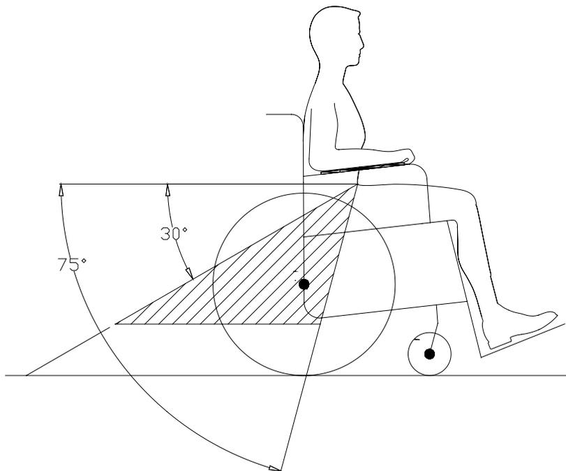
**Note:** Steeper side-view pelvic-belt angles are especially important if the pelvic belt is intended to be used for postural support in addition to occupant restraint in a frontal crash. Steeper angles will reduce the tendency for a vertical gap to develop between the user and the belt due to compliance of seat cushions and belt movement, thereby reducing the tendency for the user to slip under the belt and for the belt to ride up on the soft abdomen during normal use.
