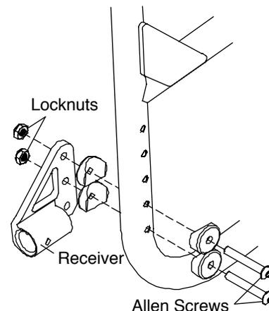
**Note:** The backrest extension may also be secured in place by these Allen screws.
