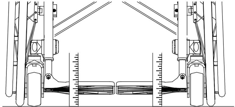
**Note:** When adjusting the height of the footrest, make sure that at least 4.5 cm of the extension tube remains up inside the frame tube. See Figure 3-4.
