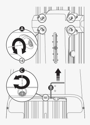
This is one way to adjust the angle of the armrest. The lower lock nut has a left-hand thread.
