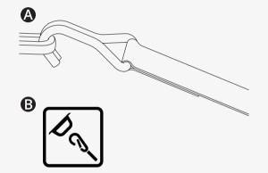
After you have secured the straps to your wheelchair, secure the other end of the straps to your vehicle according to the appropriate instructions. The end-fitting on the strap must comply with ISO 10542–1:2012, which is an international standard that governs wheelchair tie-downs and occupant-restraint systems. Every vehicle tie-down system is different, and it is important that you follow the instructions for your particular vehicle system.
