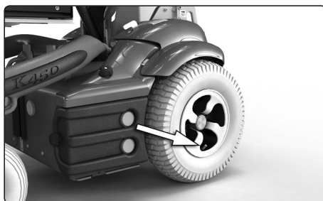
Filling valve, rear tire
