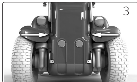
The Allen screws that attach the back cover.
