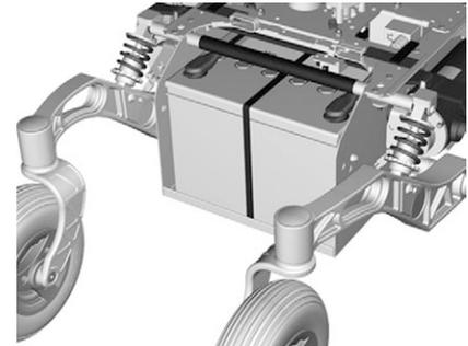
*Figure 107. Rear battery terminals*
