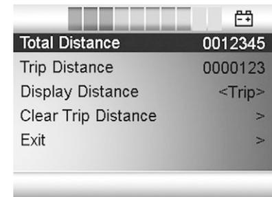
Figure 34. Distance measurement
