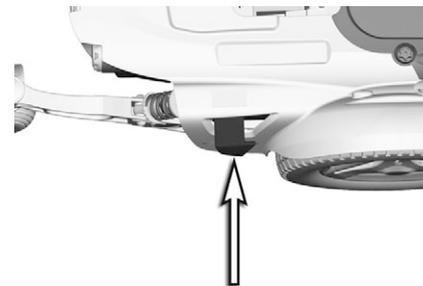
*Figure 92. Resetting released brakes*
