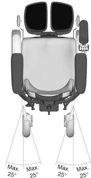
*Figure 98. The angle of the loading straps must not exceed 25 degrees.*
