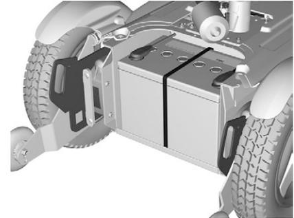
*Figure 106. Front battery terminals.*
