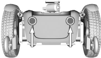
*Figure 3. Front Reflectors*
