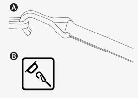
After you have secured the straps to your wheelchair, secure the other end of the straps to your vehicle according to the appropriate instructions. The end-fitting on the strap must comply with ISO 10542–1:2012, which is an international standard that governs wheelchair tie-downs and occupant-restraint systems. Every vehicle tie-down system is different, and it is important that you follow the instructions for your particular vehicle system.
