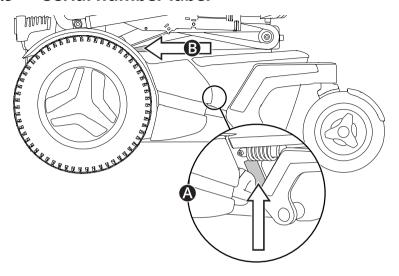
The serial number label is located on the lower, left side of the wheelchair chassis. An additional serial number label is located on the seat lift. You may need to lift the seat for better visibility.
