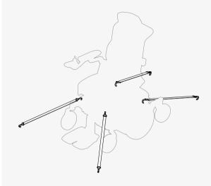
You must use both pelvic-belt restraints and shoulder-belt restraints. Make sure that the belt restraints are as tight as possible, without becoming uncomfortable, and that they are not twisted. They must be close to your body and not held away by parts of the wheelchair. Adjust your restraint system such that the release mechanisms cannot be pressed during a crash.
