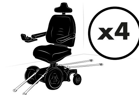
Figure 1 63. The wheelchair has four tie-down points. The wheelchair and tie-down position in this picture is generic.
