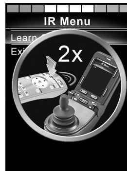
Figure 73. Point the remote control at the IR receiver. Press the button twice.
