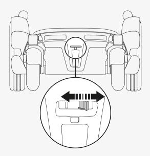
When you store for a long time, fully charge the batteries. Remember to switch off the main circuit breaker. Charge the batteries every month.
