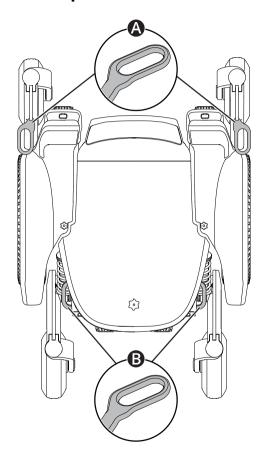
The wheelchair is equipped with four tie-down points used for transportation  $\blacksquare \times \blacksquare$ . Two in the front  $\bullet$  and two in the rear  $\bullet$ .
