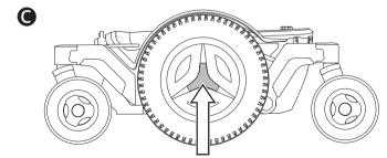
The wheelchair is equipped with reflectors at the front, the rear, and the sides.
