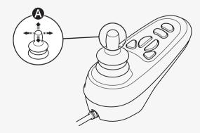
Do not move the joystick before, during, or immediately after you turn on the control system. If you move the joystick during this time, it can generate a joystick error. If this happens, turn off and then on the wheelchair.
