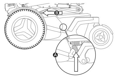
The serial number label is located on the lower, left side of the wheelchair chassis. An additional serial number label is located on the seat lift. You may need to lift the seat for better visibility.
