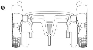
The wheelchair is equipped with reflectors at the front and rear.
