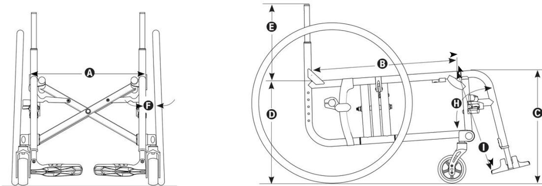
**SEAT DEPTH B** Measure from 1/2" in front of back post to the front edge of seat sling. (12"-14" Seat Depths B not available with 25" (559) and 26" (560) Rear Wheels.)
