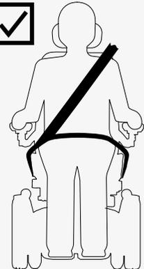
The shoulder-belt restraint should be worn over the shoulder. The pelvic-belt restraint should be worn low across the pelvis and within the preferred zone of 30° to 75°. It is desirable to have a steeper angle within the preferred zone. Make sure that the wheelchair is not lifted or tilted. The wheelchair must be in the position shown in the illustration.
