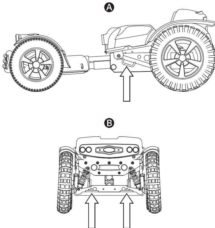
The wheelchair is equipped with four tie-down points used for transportation 🚗✈️🚚. Two on the sides **A** and two at the rear **B**.
