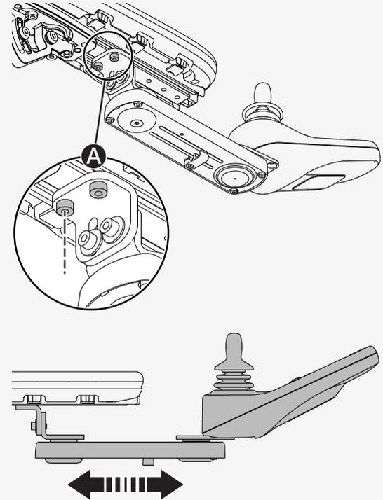
This is how you adjust the angle of the control panel.
