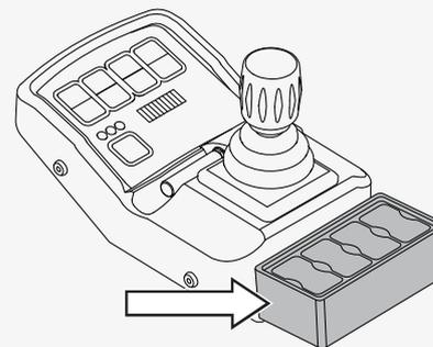
You can enable and disable the joystick menu. To enable it, press and hold the lights button and the right turn indicator button when you turn on the wheelchair. Three beeps indicate that the joystick menu is enabled. Turn off the wheelchair and repeat the process to disable the joystick menu. Two beeps indicate that the joystick menu is disabled.
