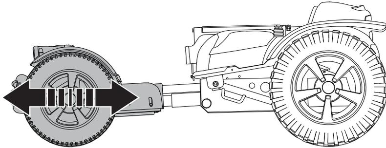
The seat control panel controls the power footplate extension.
