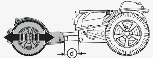
Put the adjustment rod in the preferred position. The measurements below indicate the distance between the centre of the front and rear wheels.
