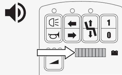
Seat rotation out and seat lift pinch protection active Error code: LED 3 flashes. If pinch protection is active, the seat lift cannot be lowered.
