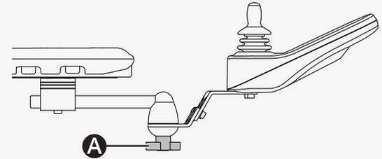
You can angle the rotational control panel to either side. This is how you adjust the angle.
