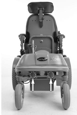
*Figure 4. Rear Lights and Reflectors.*
