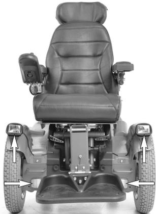
*Figure 3. Front Lights and Reflectors.*
