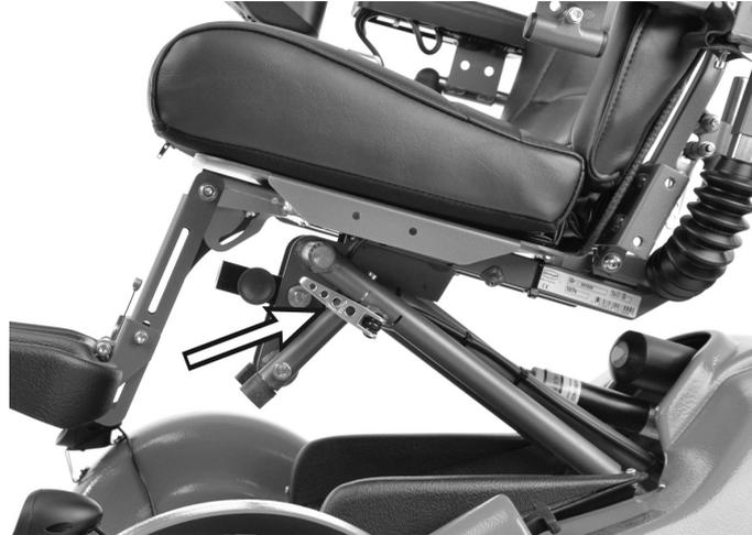
*Figure 12. Seat angle quick-acting lock.*
