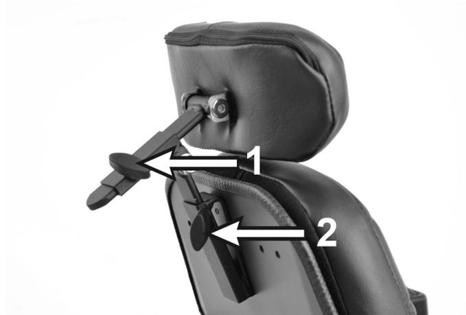
Figure 20. Head rest adjustment
