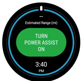
1 With your SmartDrive MX2+ unit turned on, launch the SmartDrive MX2+ app and touch "TURN POWER ASSIST ON"
